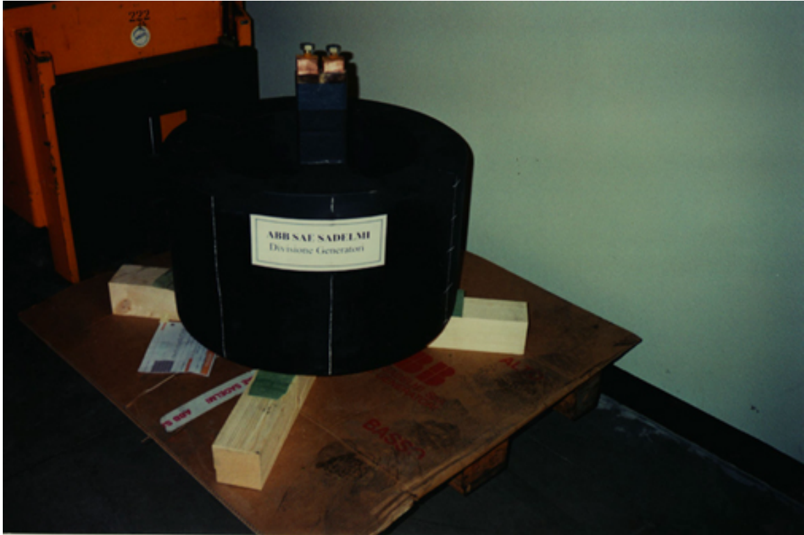
Completed prototype of the innermost coil of the central solenoid.
